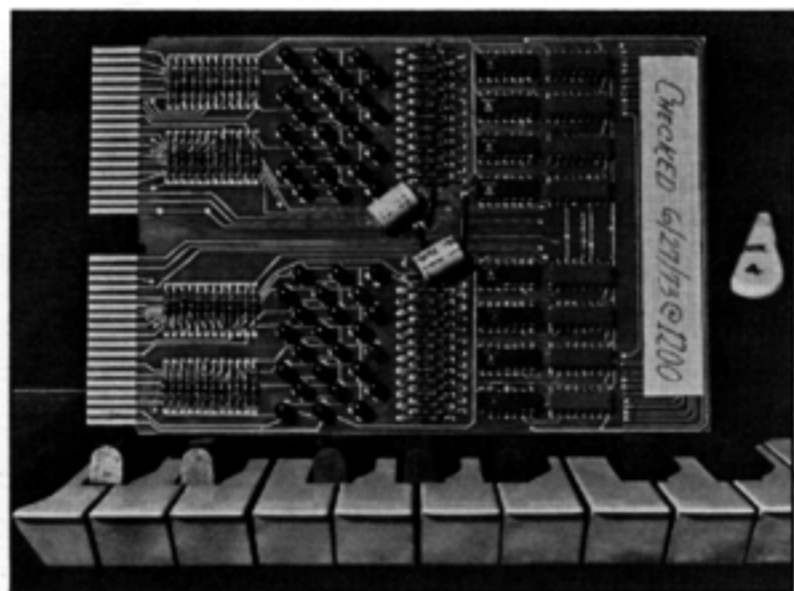
A key circuit from Knowlton's interface system.
