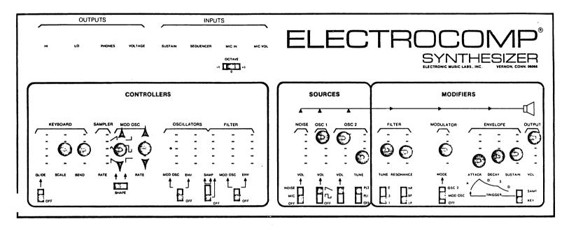
From the Modulator the audio path continues through the Voltage Controlled Amplifier (VCA). This device is not shown on the front panel, but is inside your synthesizer. It is the primary way you have of controlling loudness.
