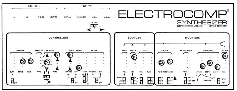
You should hear Oscillator 1's pitch varying slowly. Adjust the speed with the MOD. OSC. Frequency slider. Adjust the amount of pitch change with the MOD. OSC. slider in the located Vibrato (Oscillator).
