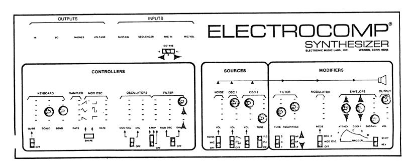
The Keyboard and Envelope control voltages occur once for each key depression. They differ from the Sampler and Modulation Oscillator which repeat a number of times during a key depression.
