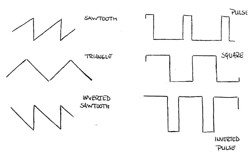
The slider provides for continuous variation from sawtooth through triangle to inverted sawtooth if the shape switch is to the left.
