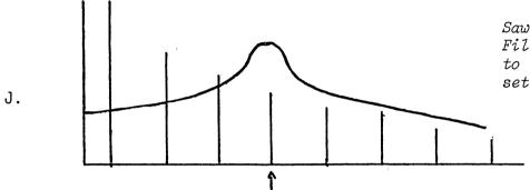
Sawtooth wave into a Band Pass Filter with the Filter "tuned" to the 4th harmonic, Resonance set Med. Before continuing to the next modifier, read the following and consider it in the context of your experimenting. Please go back and reconsider the Filter in this light.
