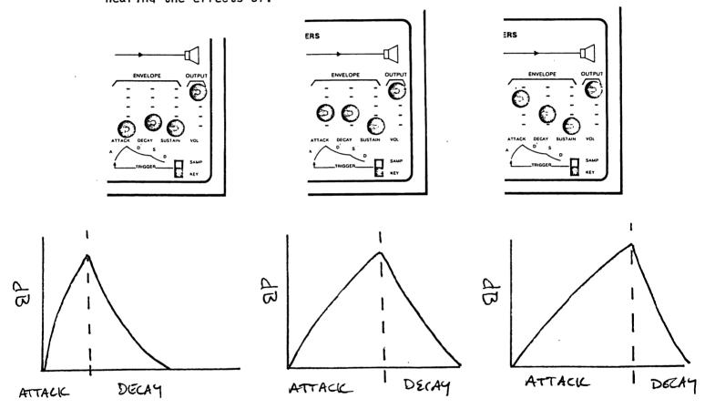
The Sustain slider has been set at maximum, reduce it to about halfway. Set the attack to zero and the Decay about halfway. Depress a key and hold. Listen.
